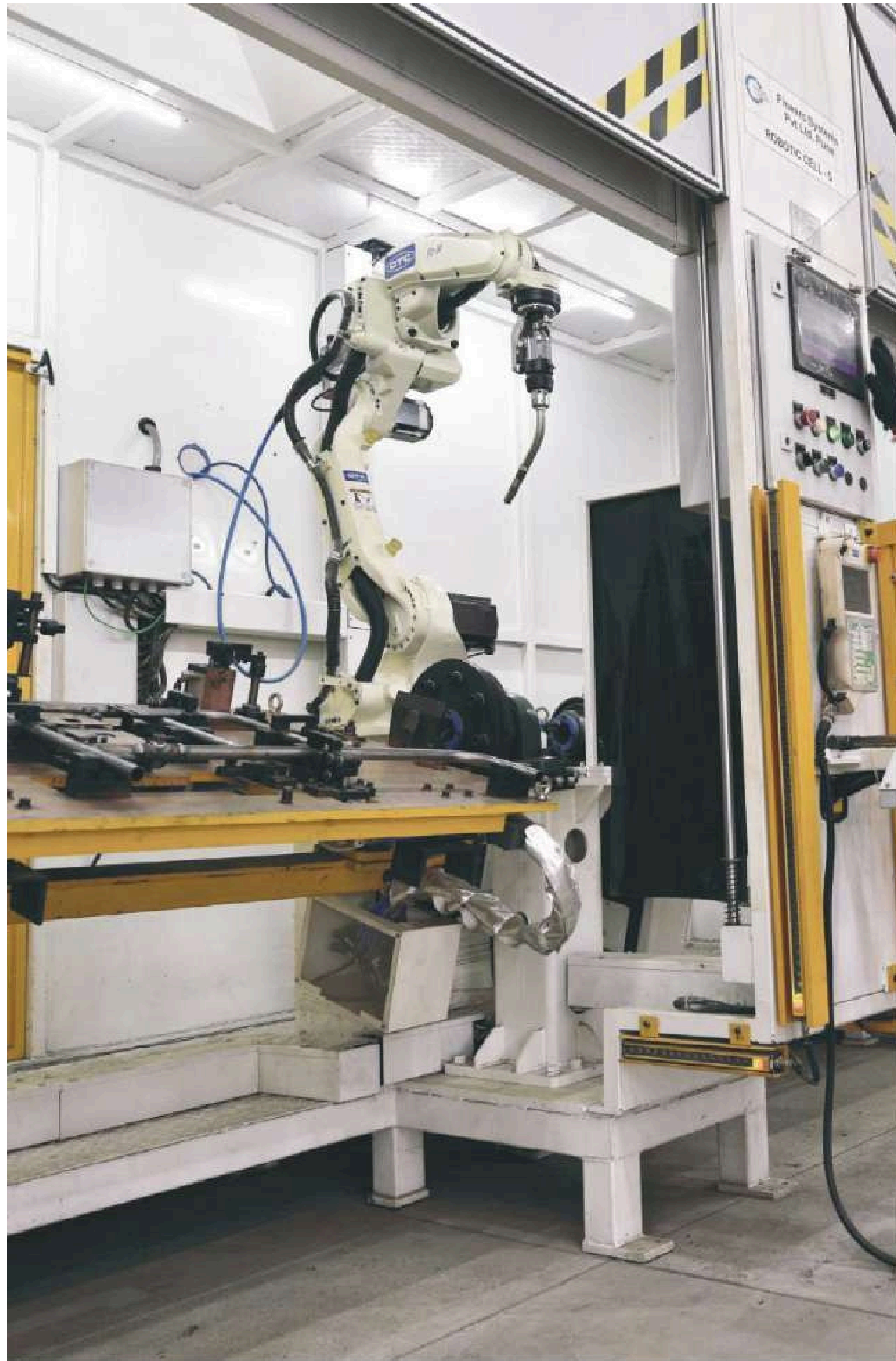
Houses Robots arranged in a sequence which are programmed to perform Mig Welding on child parts and structural frames of Wheel Chairs.
