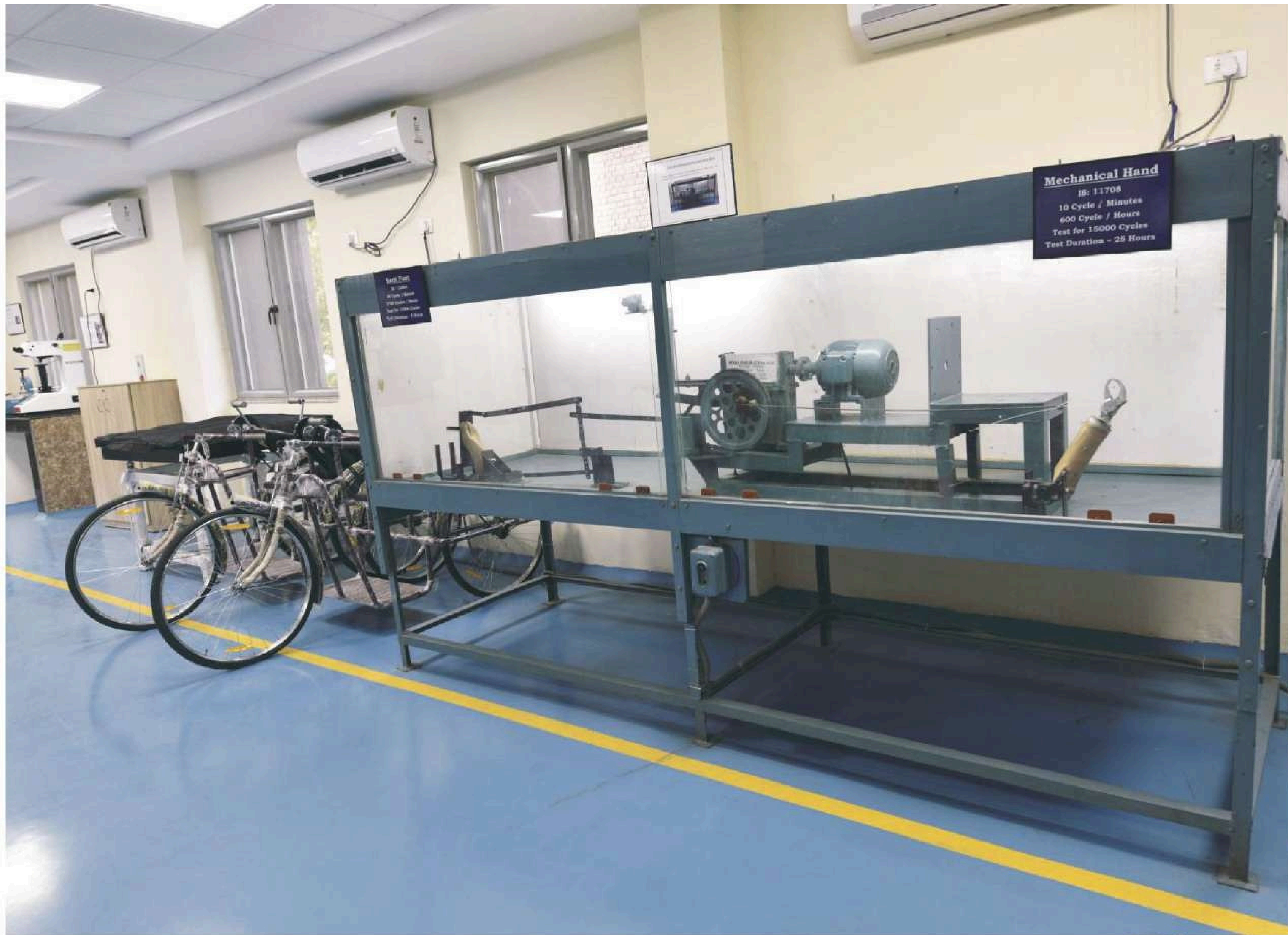
Quality test of Mechanical Hand through Cyclic Test procedure for 15000 cycle of as per IS : 11708
