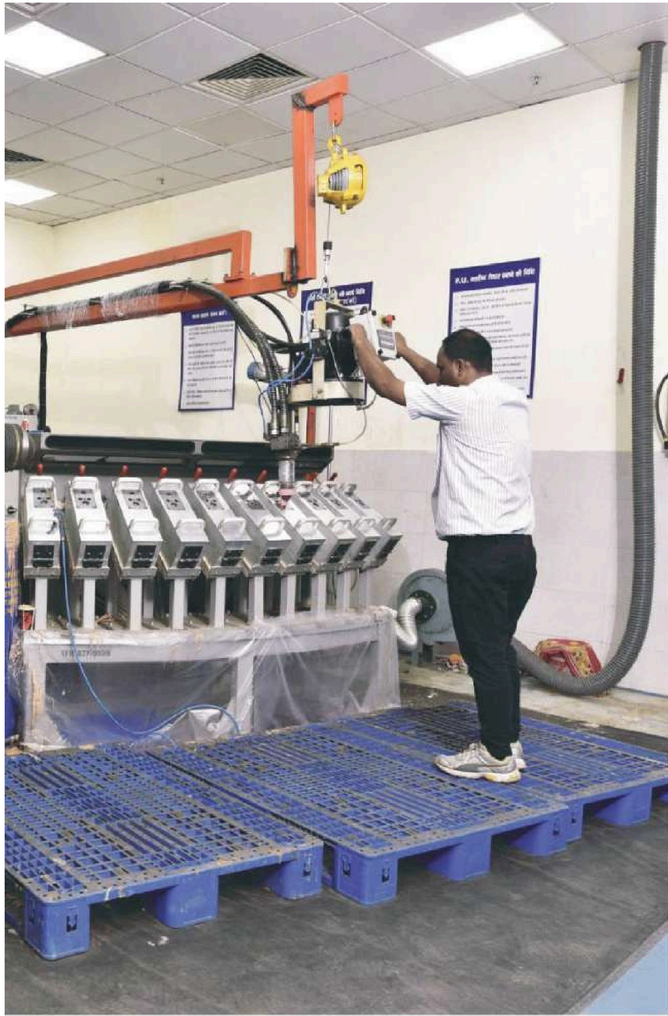
PU molding shop for SACH foot and manufacturing at high and prosthetics shop.
