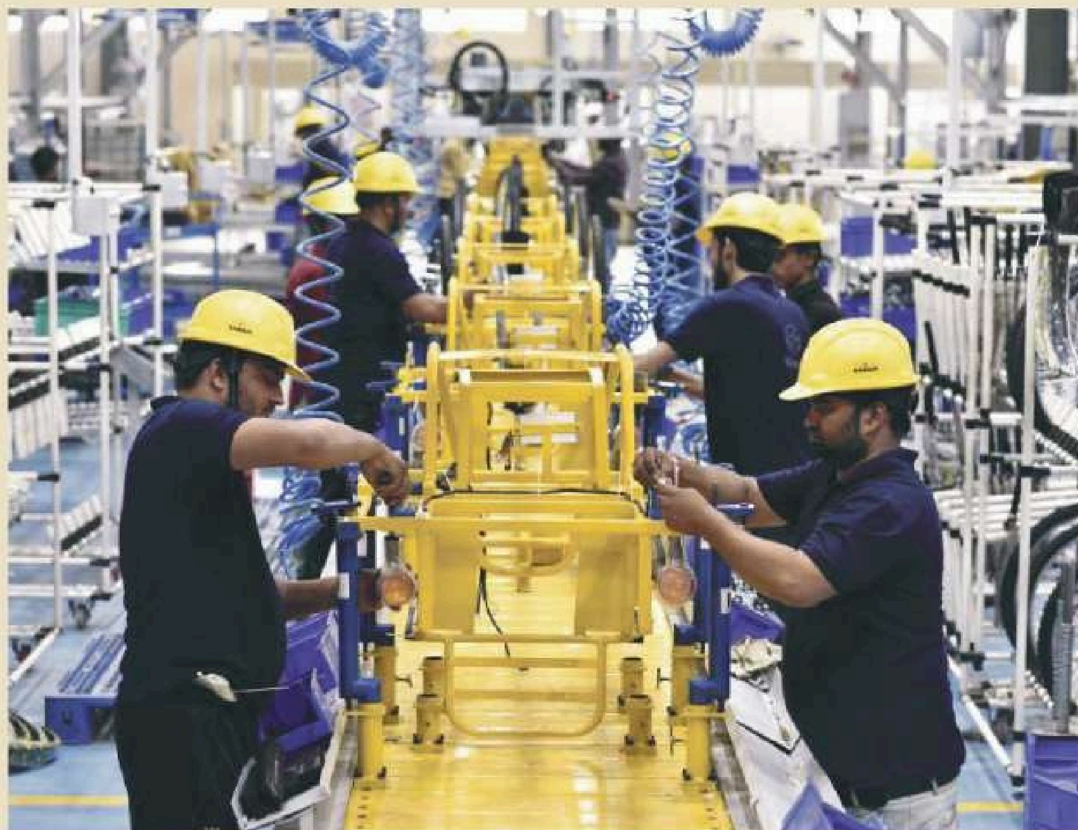
Motorized Tri-cycle assembly line on automatic conveyor system.
