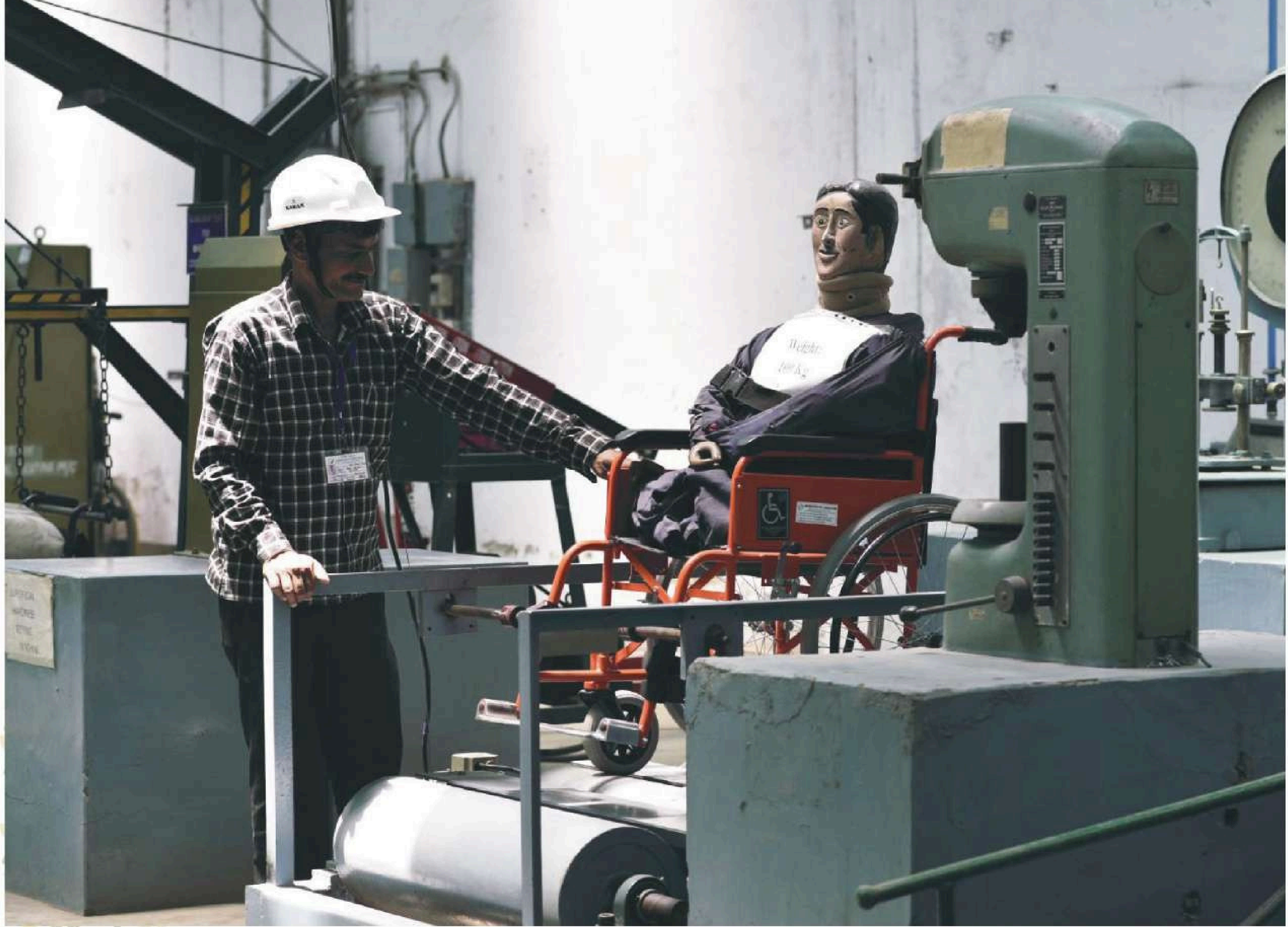
Hazard Running Test for Wheel Chair as per IS : 7454
