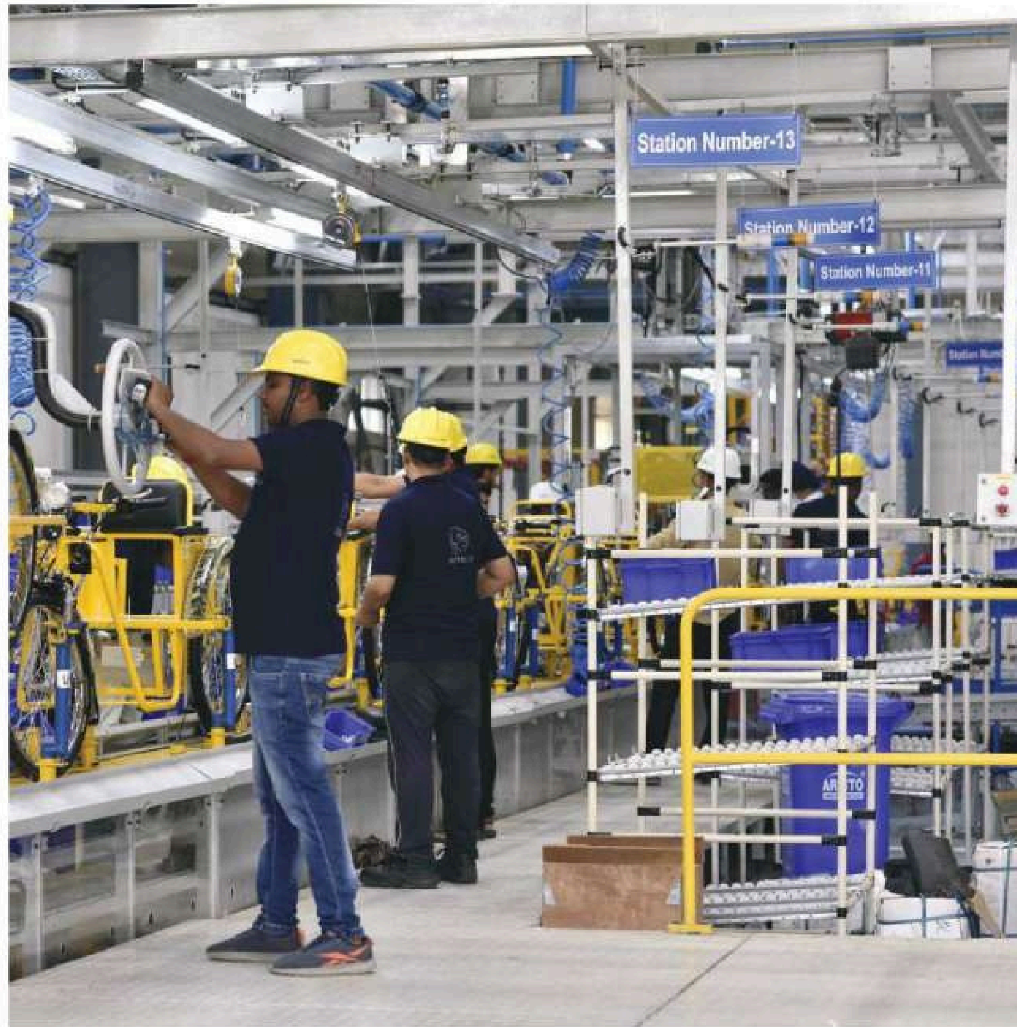
It is designed for final assemblies of Wheelchair, Motorized Tricycles and wheels. The Conveyor, lightings, Electric Panels, Work Stations, Overhead Rails have been installed.
