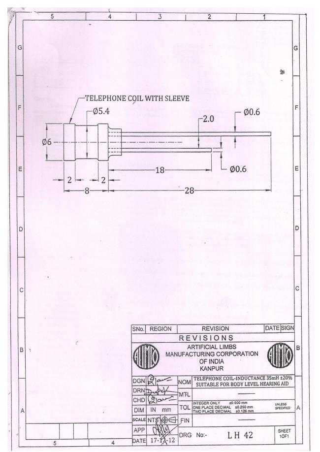
(Telephone Coil-Inductance 35Mh±20% Suitable for Body Level Hearing Aid (As per Drawing Enclosed with "Annexure A")
